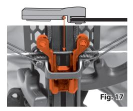
**CAUTION:** In addition to having the sled seated correctly with both string grooves fully engaged on the string, make sure that the rope is seated in the groove on the stock as shown in **Section 6C, Fig. 16**. Make sure that the rope is parallel to the rail and the rope runs unobstructed from the rope grove to the pulley wheel on the sled. Failure to make sure that rope runs unobstructed, may cause damage to the sled, the crossbow and/or cause injury to the user.
